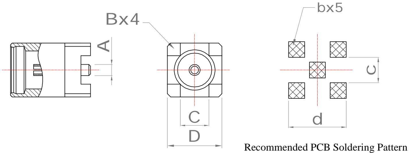
Recommended PCB Soldering Pattern
